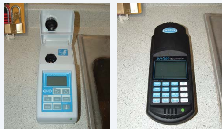
Handheld Water Quality Testing Equipment (Left to Right) Turbidimeter (measures Turbidity), Colorimeter (measures Chlorine, Iron, and Manganese)
