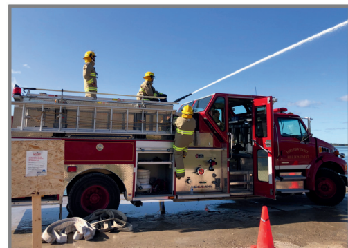
A deck gun is a nozzle fixed to the top of a fire truck (sometimes connected to hose). The pump operator opens a valve to start the water.
