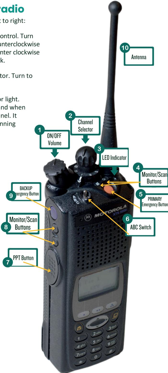
All hand-held radios have similar components but will vary from the model in this image. Make sure to use the instructions and diagram associated with the device(s) used by your fire department.
