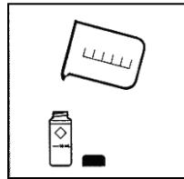
2. Add one DPD Total Chlorine Powder Pillow to the other cell. Place the cap on the cell and shake it gently for 20 seconds or until all the powder has dissolved. Wipe the cell clean of fingerprints and dust **Wait 3 minutes for the powder to react**. This will be called the '**prepared sample**'.
