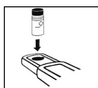
6. Tightly cover the cell with the instrument cap.
